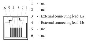
Ports La and Lb are electrically isolated from the PABX system circuit.
